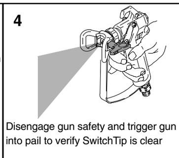
**Note:** If SwitchTip is still clogged, follow **Pressure Relief Procedure** in gun or sprayer manual, and remove SwitchTip for cleaning.
